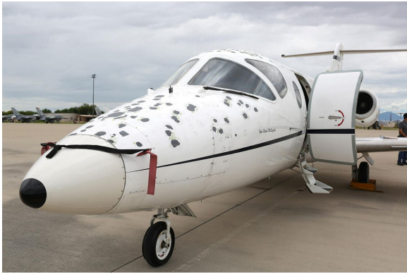
Raytheon Beechjet Hail Damage, and Pitot Covers
