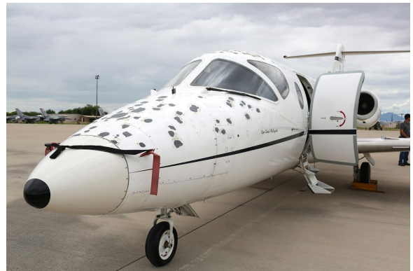
Raytheon Beechjet Hail Damage, and Pitot Covers
