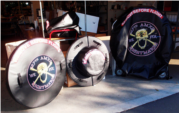
A-10 Engine Intake Plug, Exhaust Plug/Cover, Intake Cover (from left to right)
