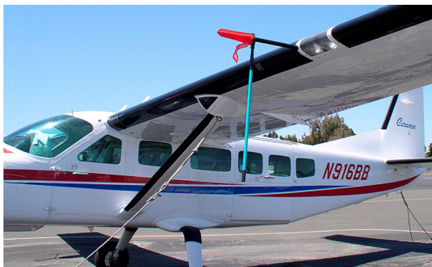
Cessna 208 Caravan Telescoping Pitot (for amphib. models)
