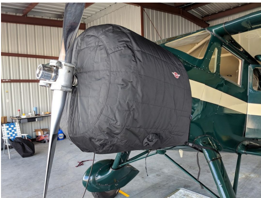
Wacon Cabin Biplane ZQC-6 Insulated Engine Cover
