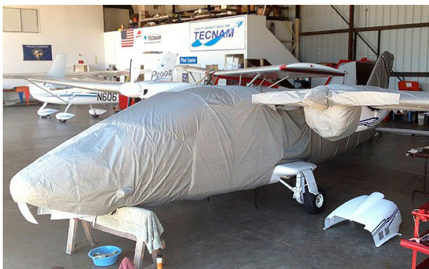
Tecnam Twin Canopy/Nose, Empennage, Wing/Engine, & Propellor/Spinner Covers
