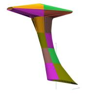
Autogyro Calidus Rotor Mast Cover, 3D model
