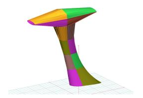
Autogyro Calidus Rotor Mast Cover, 3D model
