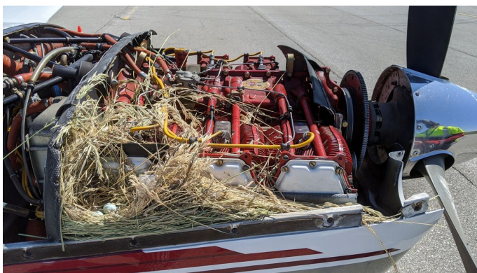
ENGINE PLUGS PREVENT BIRD NEST FOD. Piper Saratoga Engine Cowling Bird's Nest Taylorcraft Engine Inlet Plugs
