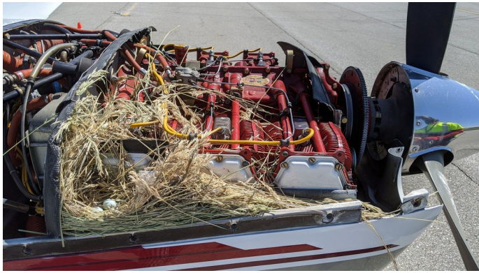
Slingsby T-67 Firefly Engine Inlet Plugs ENGINE PLUGS PREVENT BIRD NEST FOD. Piper Saratoga Engine Cowling Bird's Nest
