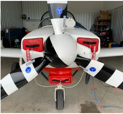
Slingsby T-67 Firefly Engine Inlet Plugs ENGINE PLUGS PREVENT BIRD NEST FOD. Piper Saratoga Engine Cowling Bird's Nest
