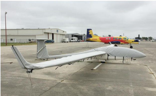
DG-505 Canopy/Nose, Wing, Empennage & Horiz. Stab. Covers End Cap Covers are used when wing are in folded position.
