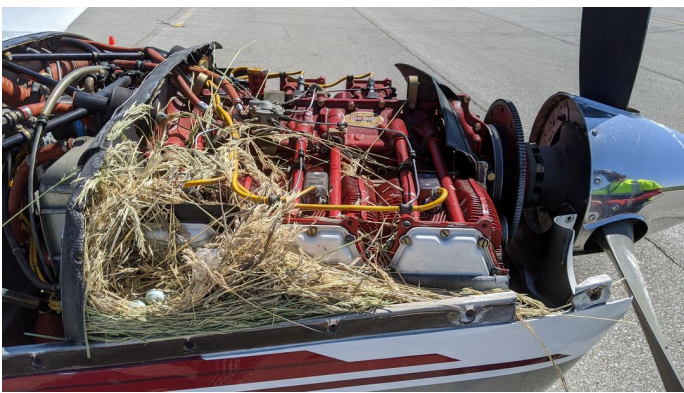
Van's Aircraft RV-7A Engine Inlet Plugs ENGINE PLUGS PREVENT BIRD NEST FOD. Piper Saratoga Engine Cowling Bird's Nest
