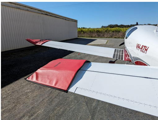
Sling TSI Horizontal Stabilizer Tip Pads
