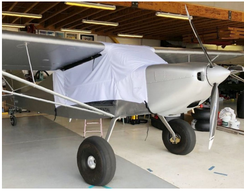
Rans S-20 Canopy Cover, test fit cover
