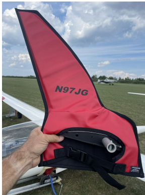
Schempp-Hirth Ventus-2B winglet/wingtip pads
