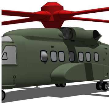
Sikorsky S-92 Main Rotor Hub Cover
