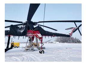
Sikorsky S-64 Canopy/Nose, Engine Area, Blade, Rotor, Tail Rotor Sikorsky S-64 Skycrane, CH-54 Tarhe Insulated Engine, Rotor Covers (illustration)
