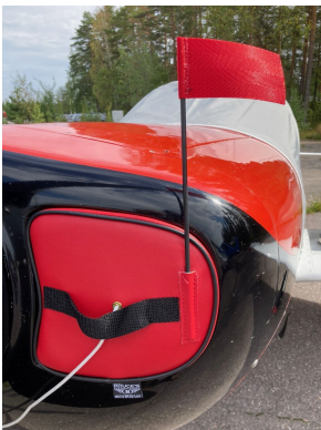
Siai Marchetti SF260 Engine Plugs ENGINE PLUGS PREVENT BIRD NEST FOD. Piper Saratoga Engine Cowling Bird's Nest
