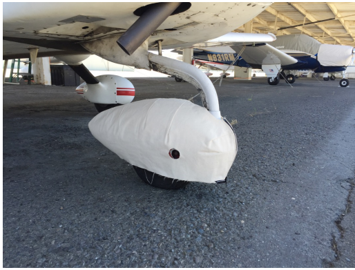
Grumman AA5 Nose Wheelpant Cover, test fit
