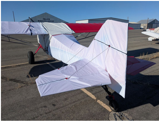
Rans S-20 Raven Canopy Cover, Wing Covers & Empennage Cover (some test fit)
