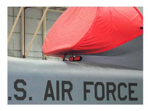
Intake Cover with small inlet plug
