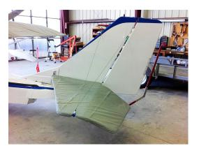
SeaRey Horizontal Stab. Cover (test fit cover)
