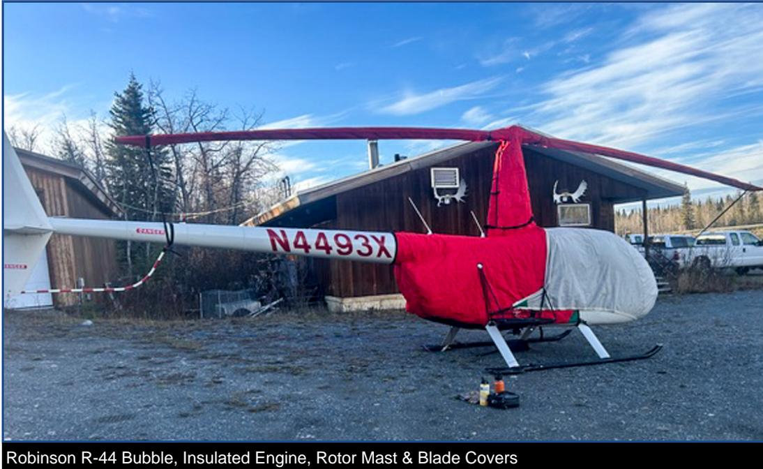
Robinson R-44 Bubble, Insulated Engine, Rotor Mast & Blade Covers
