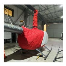
Robinson R-44 Bubble, Rotor Hub, Tail Rotor Covers, & Blade Tie-Downs Robinson R-44 Insulated Rotor Mast & Engine Covers
