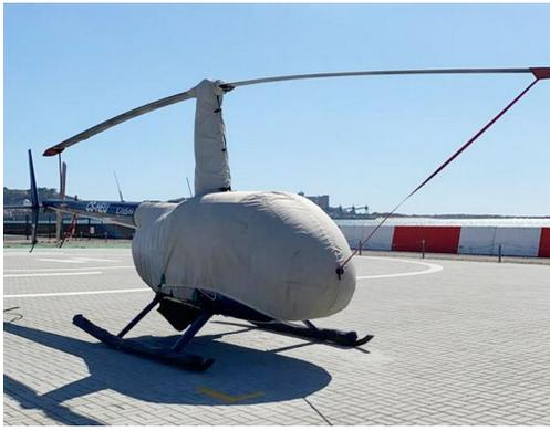
Robinson R44 Bubble, Engine, Rotor Mast Covers
