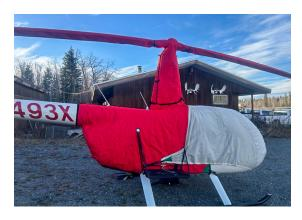
Robinson R-44 Bubble, Insulated Engine, Rotor Mast & Blade Covers
