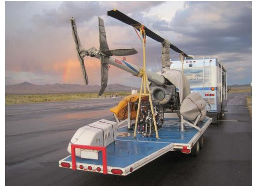
Robinson R-22 Bubble, Rotor Mast, Tail Rotor & Tail Fin Covers
