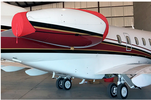
Premier Intake Plugs, Intake Covers, Pitot Covers & Cockpit HeatShields Intake/Exhaust Covers, 3-Strap Type. Successfully installed by two crew, one ladder.
