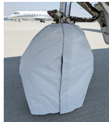
CJ1 Nose Gear Tire Cover, test fit
