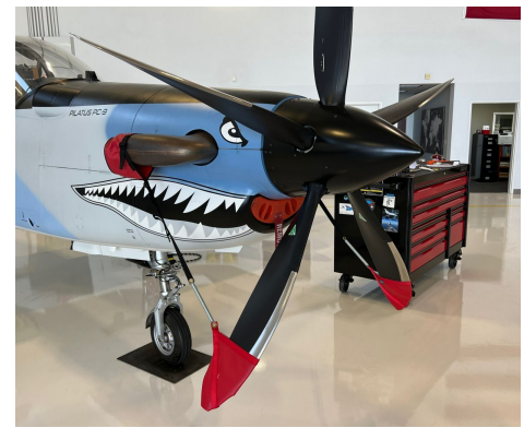
Pilatus PC-9 Prop Ties, Exhaust Covers
