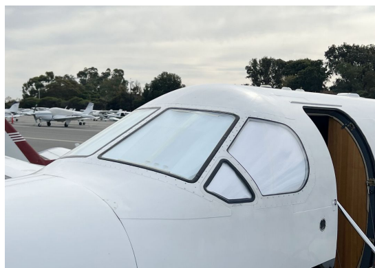
Pilatus PC-12 Cockpit HeatShields
