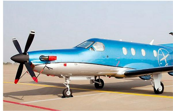
Pilatus PC-12 Engine Plugs, Prop Ties, Cockpit HeatShields
