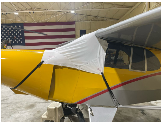
Piper J5A Windshield/Skylight Cover, test fit
