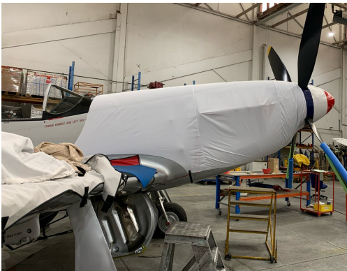
North American P-51 Mustang Canopy Cover, Belly Scoop and Chin Scoop Plugs North American P51 Engine Cover, test fit cover
