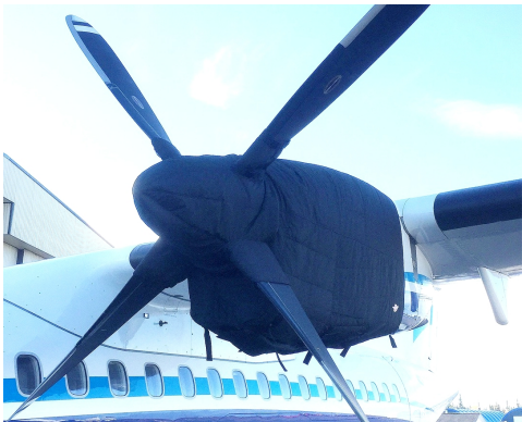
ATR-72-202 Insulated Engine & Prop Hub Covers
