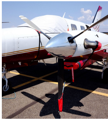
Piper Cheyenne Cockpit Cover, Engine Plugs, Prop Tie/Exhaust Covers
