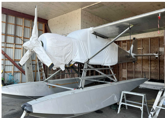
Murphy Moose Extended Canopy Cover, Engine & Prop Covers, test fit covers. Murphy Moose Extended Canopy Cover, Engine & Prop Covers, test fit covers.
