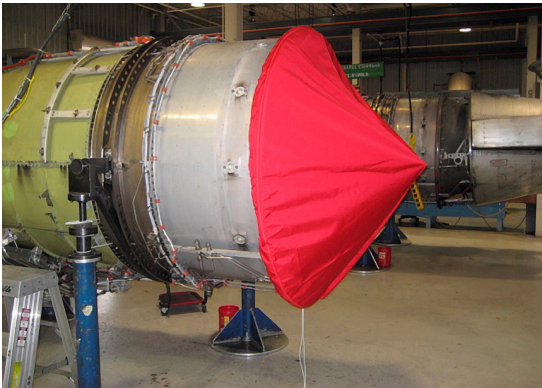
PW JT8D Off-Link Engine Shower Cap Cover Set MD-80 JT8D Intake Plugs, Solid Foam folding type& Mesh Center folding type
