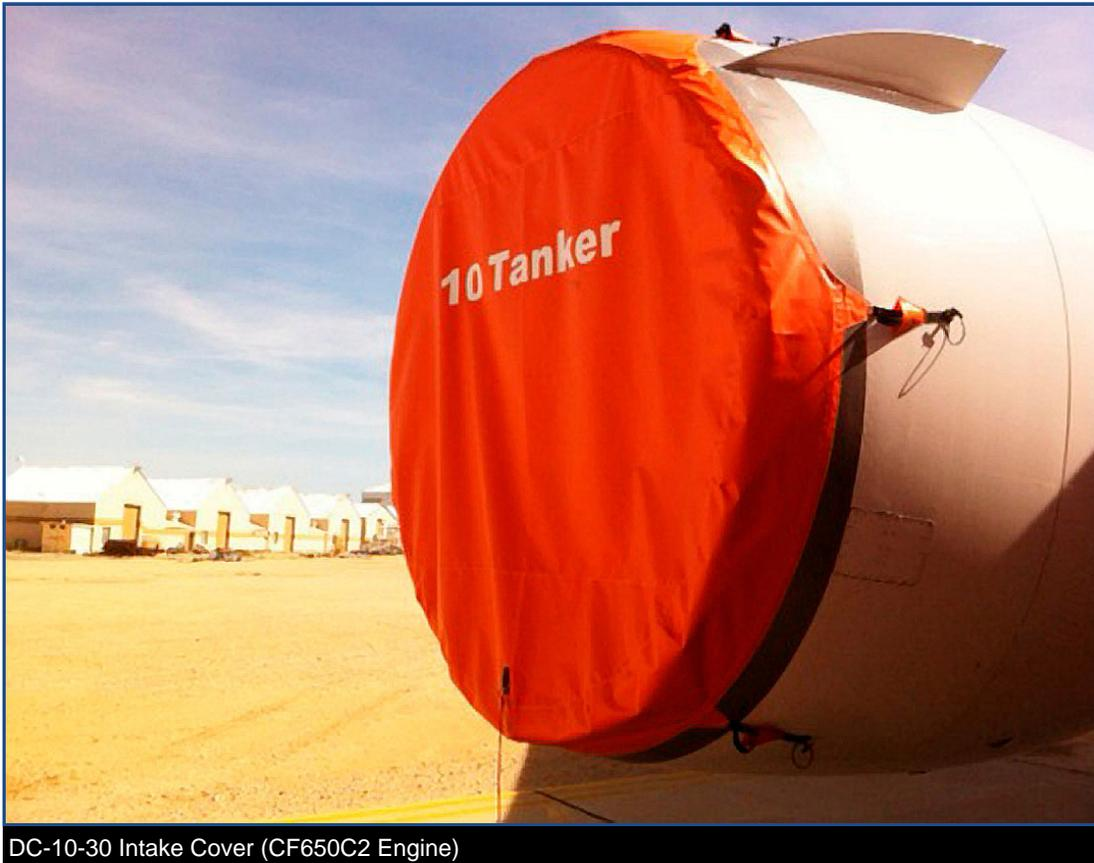
DC-10-30 Intake Cover (CF650C2 Engine)
