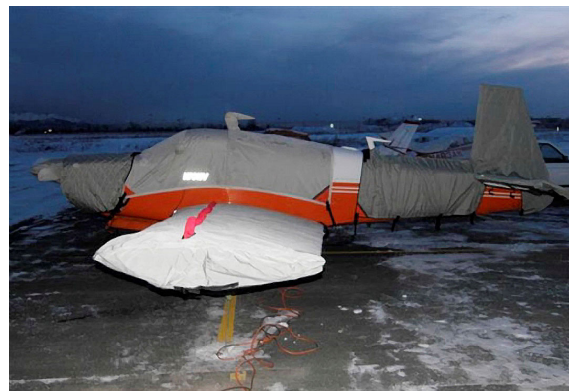
Mooney Prop/Spinner, Insulated Engine, Wing, Canopy and Empennage Covers
