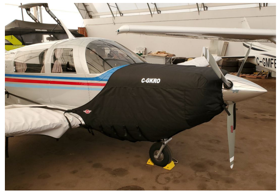
M20K 231 Insulated Engine Cover, fully enclosed
