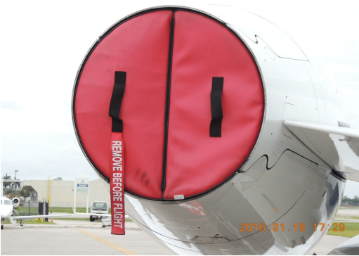
Embraer Legacy 500 Engine Exhaust Plug, folding type
