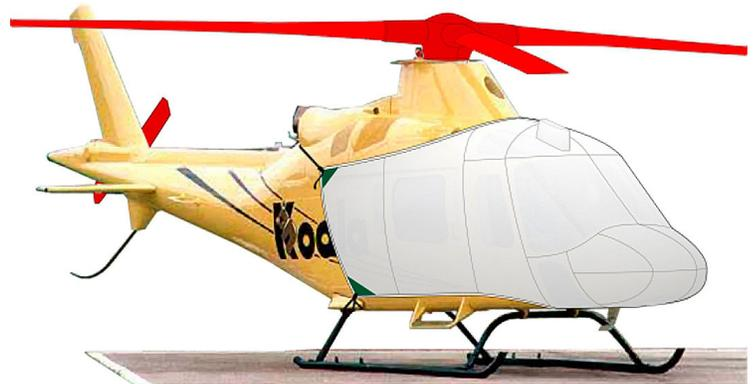
Koala Bubble, Rotor Hub, Blade & Tail Rotor Covers (illustration)
