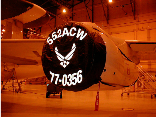
Intake/Exhaust Covers, soft type, TF-33 Engines
