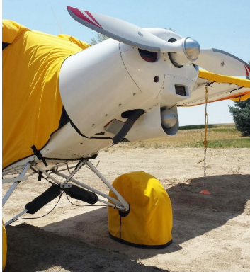
Piper PA-18 Super Cub Extended Canopy Cover, Wing & Tire Covers Cub Crafters CC19 Oversize Tire Covers, test fit cover
