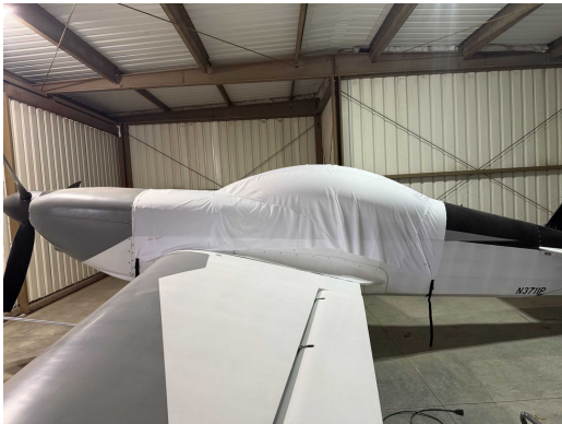
IAC One Design DR-109 Canopy Cover, test fit
