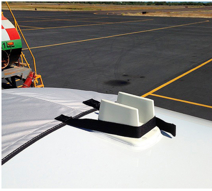
Phenom 100 EMB-500 Cockpit Cover (includes straps to hook around traffic antennae so the cover will not slip forward)
