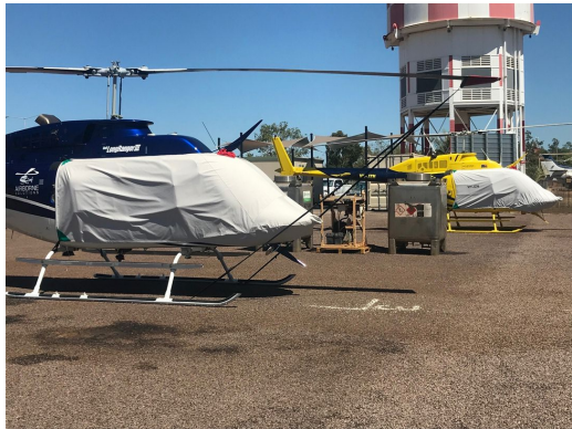
Bell JetRanger 206B and LongRanger206L Bubble Covers Bubble Cover (shortened), Engine Area Cover & Rotor Mast Cover
