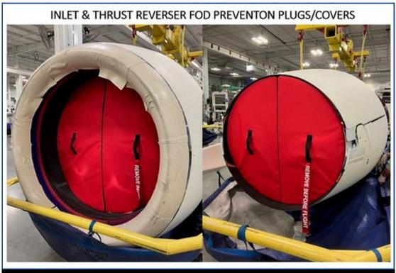
Gulfstream G500 FOD protection plugs for mfg process
