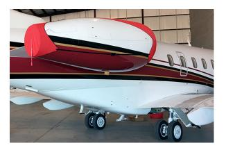
Challenger 300 Intake/Exhaust Cover Set, 3-strap Intake/Exhaust Covers, 3-Strap Type. Successfully installed by two crew, one type ladder.
