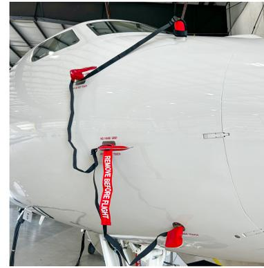
Grumman Gulfstream V, VI, VII (C-37A), G450, G550, G600, G650 Pitot Probe/Aoa Set, Heat Resistant Type (G-V And Up)
