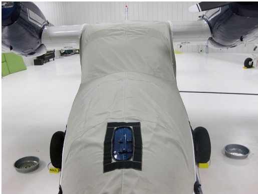
Grumman Widgeon Cockpit/Nose Cover, tie-down cleat detail
