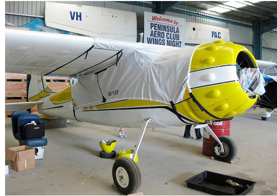
Cessna 195 Canopy Cover, over-top, 24" fwd ext to cover cowl ring gap, gas cap ext.
