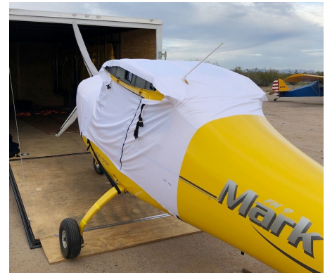
FK-Lightplanes FK-9 Canopy Cover, test fit cover
