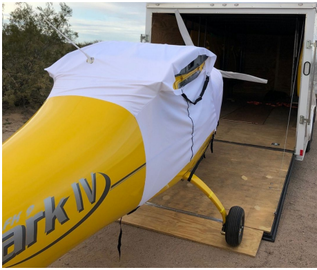
FK-Lightplanes FK-9 Canopy Cover, test fit cover
