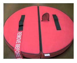
Falcon Center Engine Intake Plug
