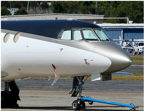
Dassault Falcon 50 Cockpit HeatShields
