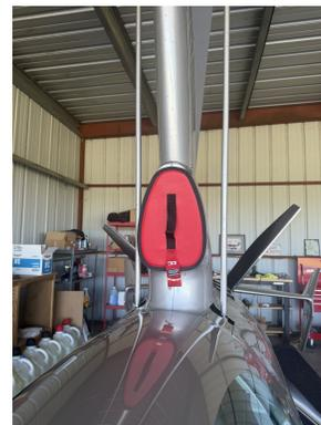
ELA Eclipse EVO Rotor Mast Inlet Plug
