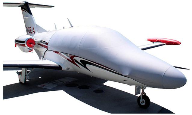
Customized to end before main antenna, with easy to use flat-hook straps.
