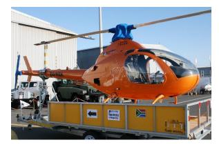
Rotorway Exec Rotor Mast and Tail Rotor Covers
