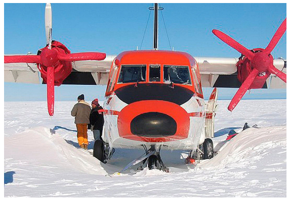
Casa 212 Insulated Engine & Propellor/Spinner Covers
